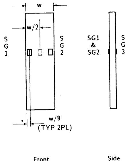
**FIG. 1 Gage Locations for System Alignment Check Coupon**
